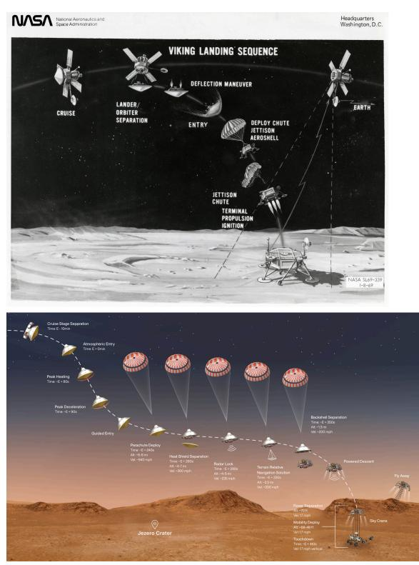
Illustrations of the Entry, Descent, and Landing (EDL) sequences for Viking in 1976, and Perseverance in 2021. Despite the wide gap between these missions in terms of technology, they both performed their landing maneuvers automatically, since our planets are too far apart to allow Earth-based engineers to control them in real time! (NASA/JPL/Caltech)
